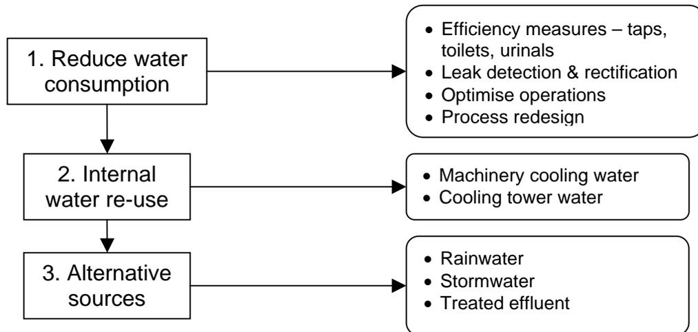
Figure 5. Schematic of Hierarchical Approach
