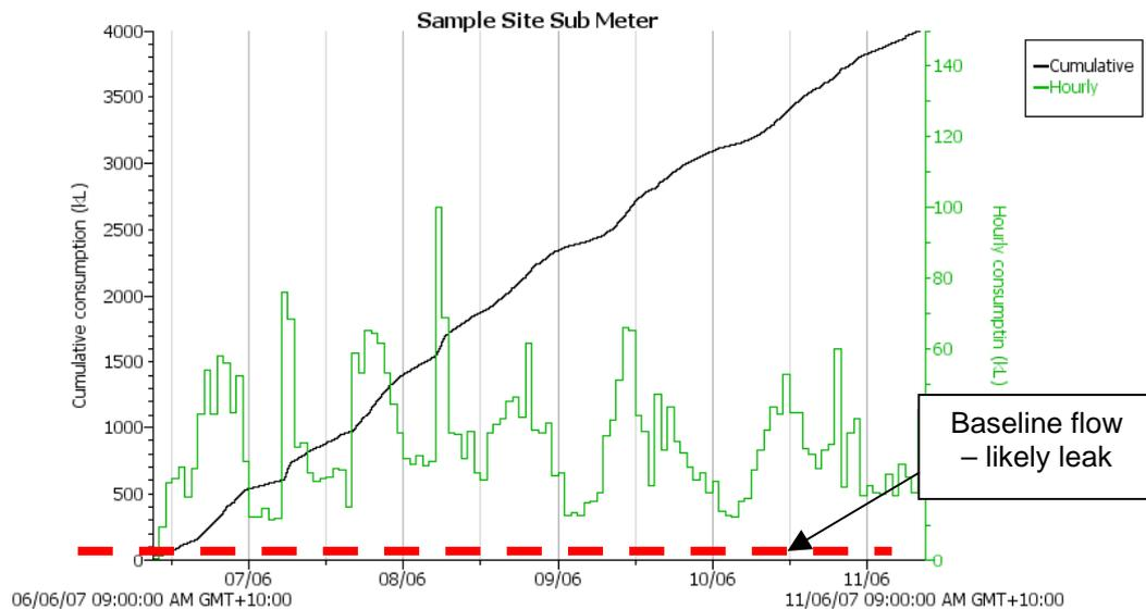
Figure 2. Sample of Temporary Smart-Metering output showing high baseline flows
