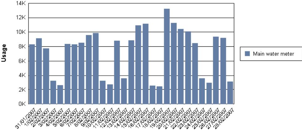
Figure 1. Sample of Daily Use measured by Smart Meter at a Large Site
