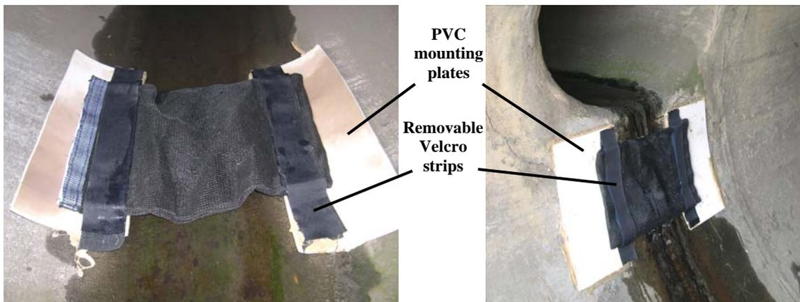
**Figure 1. Monitoring bag fitted inside drain****Figure 2. Monitoring bag fitted below drain**
