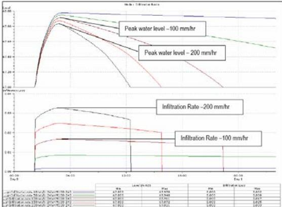
Figure 7 – Effect of infiltration rate on pond level
