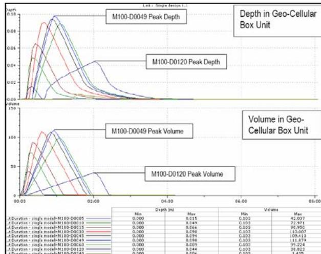
Figure 2 – Depth and volume in pervavoid unit during a constant rainfall event.
