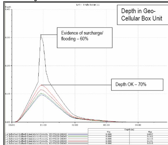
Figure 4 – Change in depth as porosity reduces.
