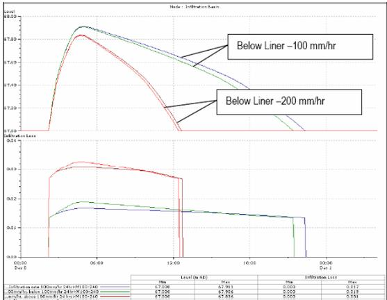
Figure 8 – Effect of changing infiltration rate below and above the liner
