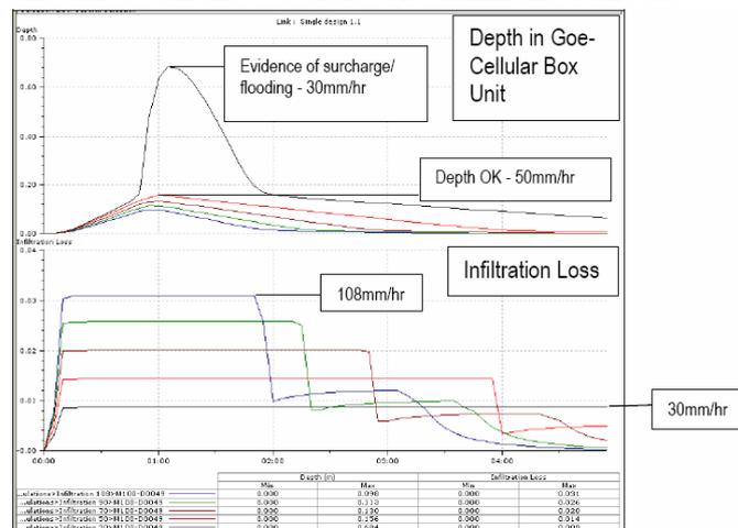
Figure 3 – Change in depth as infiltration rate changes.
