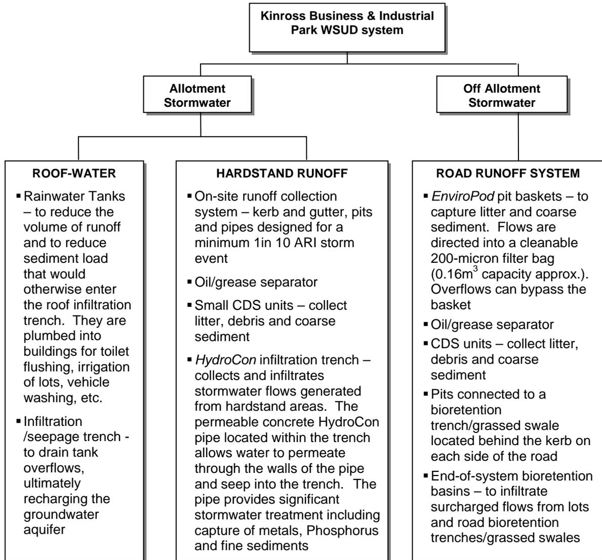
Figure 2. WSUD sub-system and their components which comprise the Kinross WSUD treatment train.
