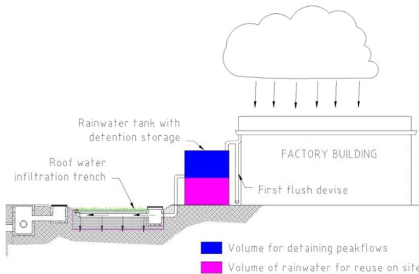
Figure 5. Roof water system of allotments
