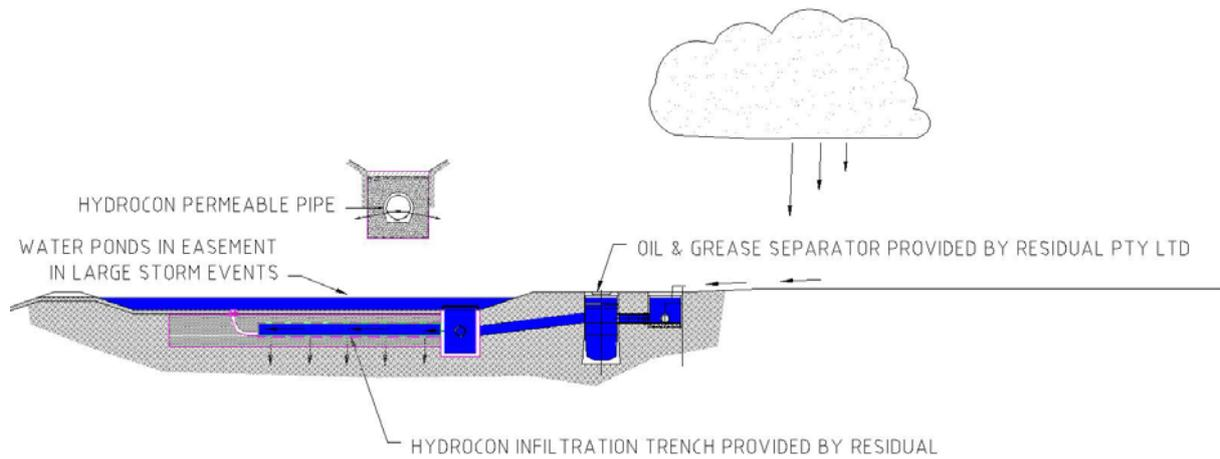
Figure 4. Lot treatment system for hardstand runoff (similar configuration used on roads)
